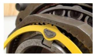
Retainer Tab Entering Groove in Nut.
