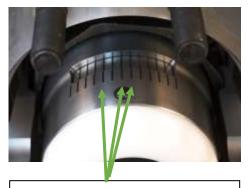
The Two Sets of Hash Marks are Aligned.
