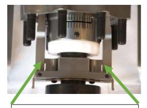
CORRECT- inside surface of both load arms in contact with edges of load arm stops.
