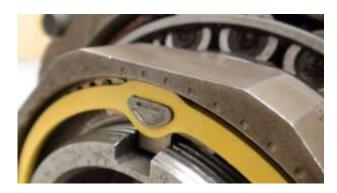
Retainer Tab Inserted Correctly in Nut.
