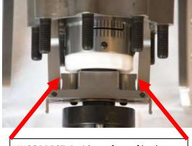
INCORRECT- inside surface of both load arms NOT in contact with edges of load arm stops.
